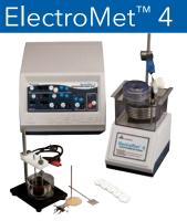
ElectroMet 4 includes ElectroMet 4 Power Source, Polishing Cell and Etching Cell. Products not available in Europe
